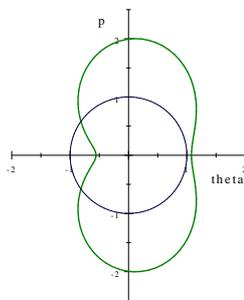
**Fig. 2.** Pressure variation distribution around the pile. Inward curve of the circle: positive change; external, negative.
