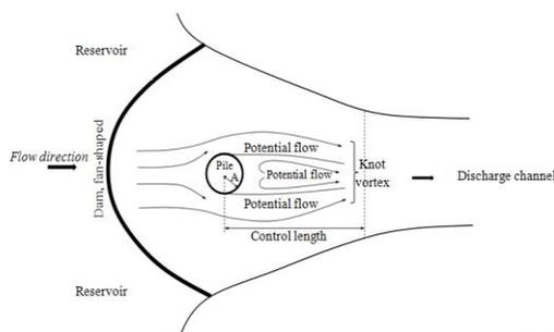
**Fig. 1.** Flow control downstream of a dam by means a pile (plan view). Flow zones and characteristics lengths are shown.
